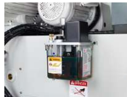
Automatic lubricator Delivers frequent lubrication oil to the caterpillar chain
