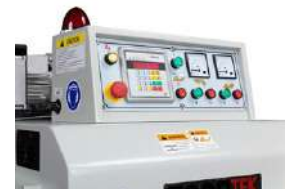
Digital positioning control The thickness of cut can be controlled by a digital positioning control.
